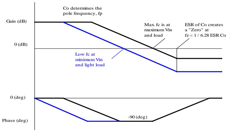
Figure 2- Control-to-Output transfer function of DCM boost converter, Gain/phase corresponding to low  $V_{IN}$  and light load are shown in blue.
