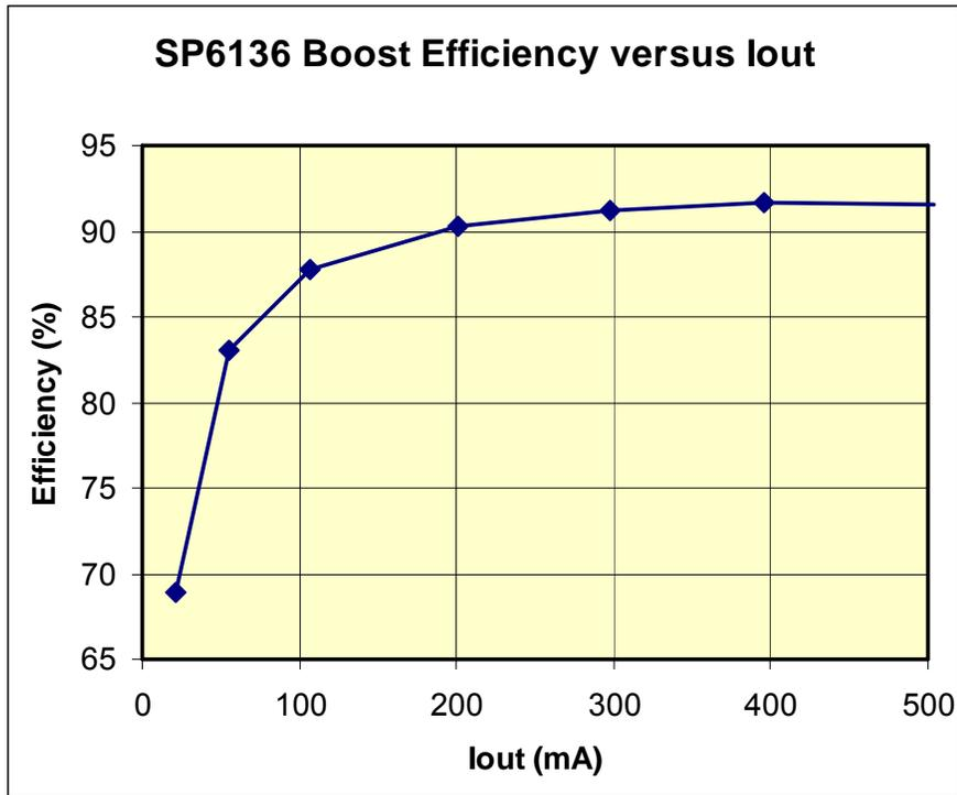
Figure 5- Efficiency at V<sub>IN</sub>=12V
