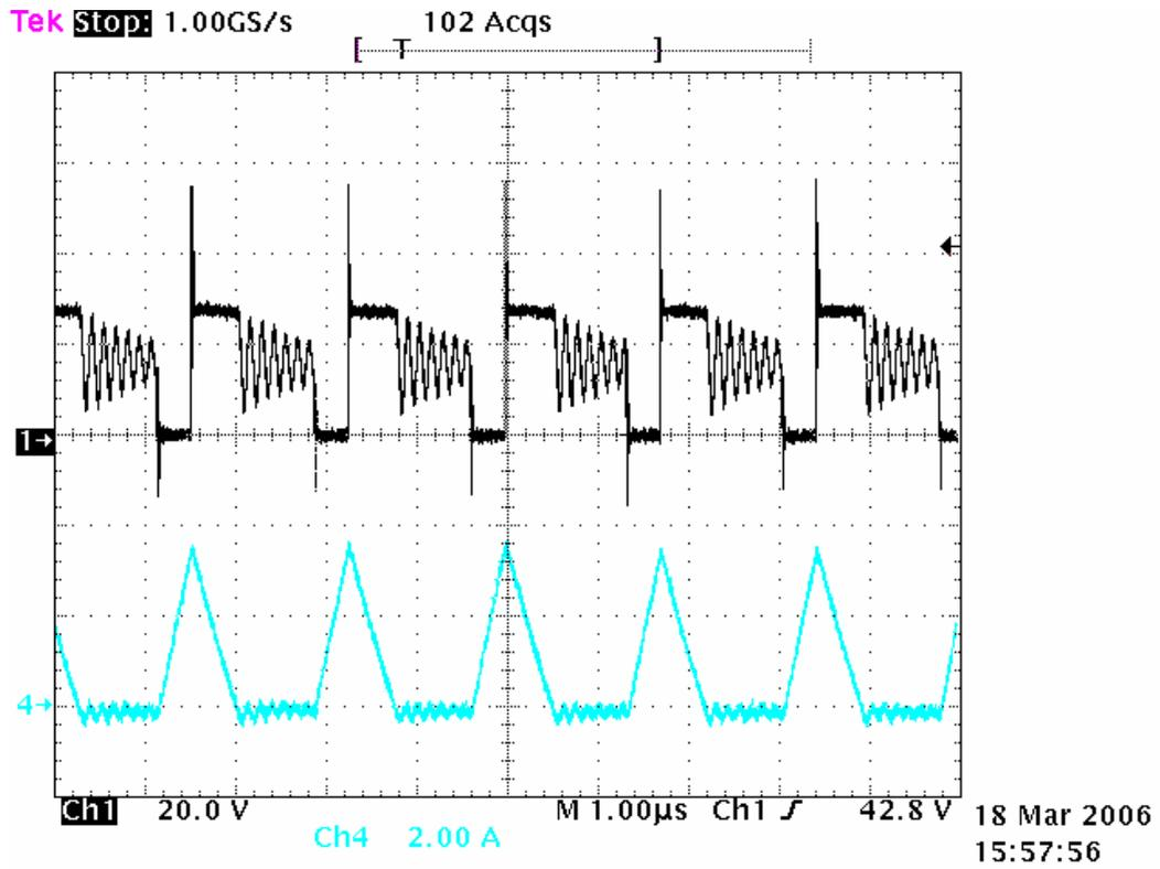
Figure 9- Converter waveforms at  $V_{in}=18V$ ,  $I_{OUT}=500mA$ , Ch1=SWN, Ch4=IL
