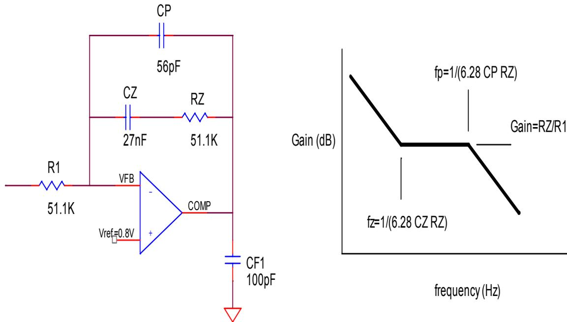
Figure 4- Error Amplifier (EA) and its transfer function for type II compensation, components shown are redrawn from figure 1, Error Amplifier is internal to SP6136 controller.
