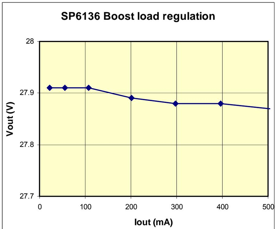
Figure 6- Load regulation at V<sub>IN</sub>=12V
