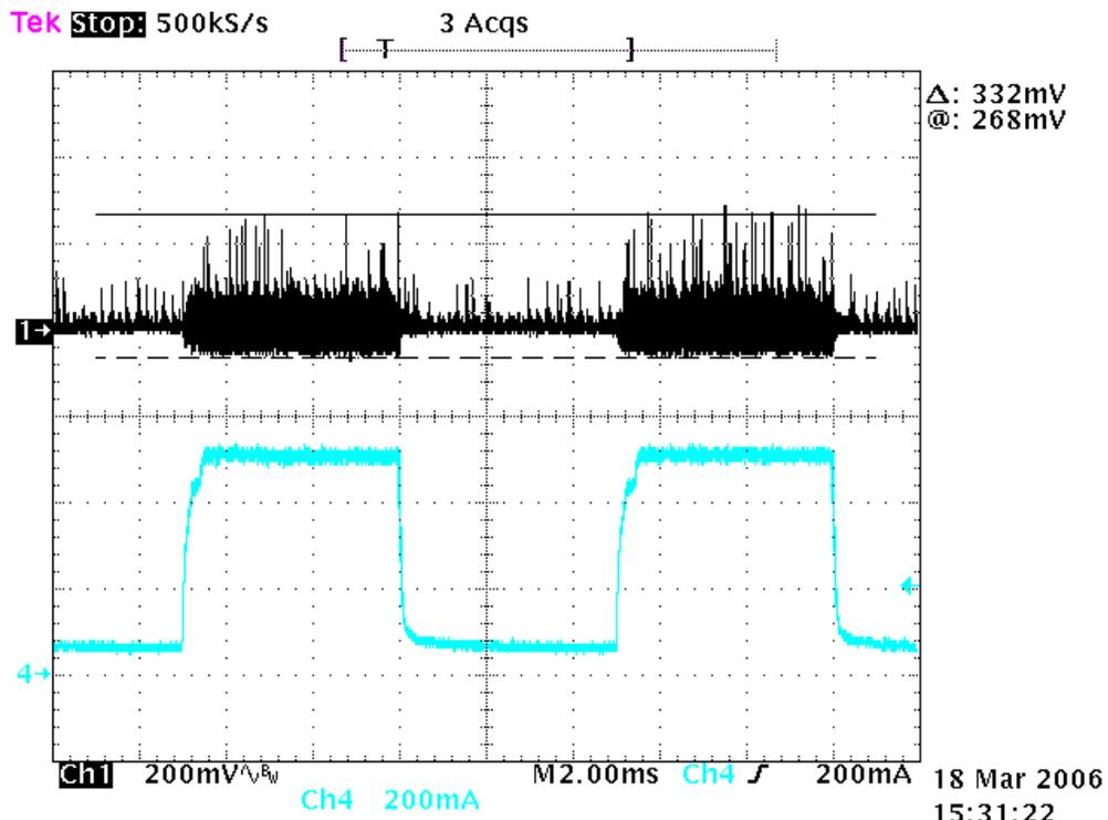
Figure 7- Step load response,  $I_1=50\text{mA}$ ,  $I_2=500\text{mA}$ ,  $f=1\text{KHz}$ ,  $D=0.5$ ,  $\text{Ch1}=\text{V}_{\text{OUT}}$ ,  $\text{Ch4}=\text{I}_{\text{OUT}}$
