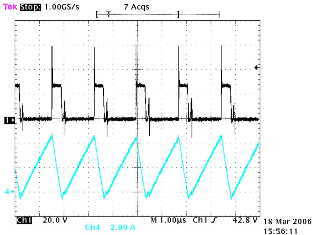
Figure 8- Converter waveforms at  $V_{\text{IN}}=7\text{V}$ ,  $I_{\text{out}}=500\text{mA}$ ,  $\text{Ch1}=\text{SWN}$ ,  $\text{Ch4}=\text{IL}$
