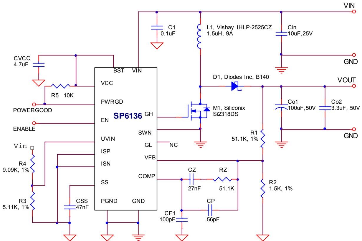
Figure 1- Boost converter based on SP6136,  $V_{IN}=7$  to  $18V$ ,  $V_{OUT}=28V$ ,  $I_{OUT}=0$  to  $0.5A$ , converter operates at Discontinuous Current Mode under all line and load conditions
