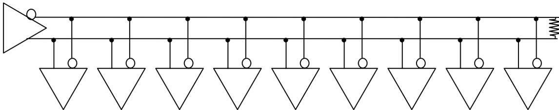
In this topology there is only one driver sending to one or more receivers. One termination resistor is recommended at the extreme end of the bus to eliminate reflections. Up to 10 receivers are permitted under RS-422 and up to 32 unit loads in RS-485. However the number of nodes can extend to much higher numbers in some configurations.
