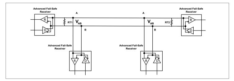
Figure 7: Advanced Fail-Safe Receiver Typical System Connections
