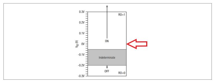
Figure 6: Advanced Fail-Safe Receiver Input Sensitivity Range
