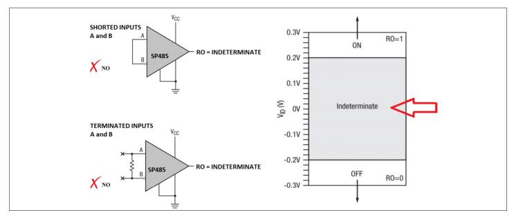
Figure 2: Standard Fail-Safe Receiver with Shorted and Terminated Inputs
