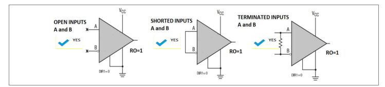
Figure 5: Advanced Fail-Safe Receiver Support of Open, Shorted, and Terminated Inputs
