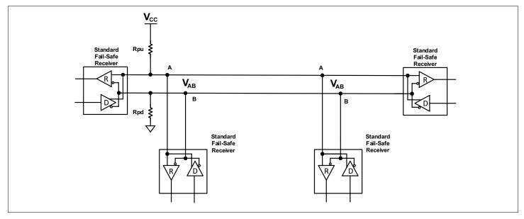
Figure 3: Bus in Idle Condition
