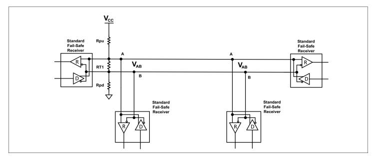
Figure 4: Standard Fail-Safe Receiver with Termination Resistors Network
