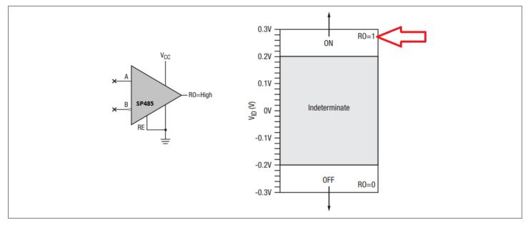
Figure 1: Standard Fail-Safe Receiver with Open Inputs
