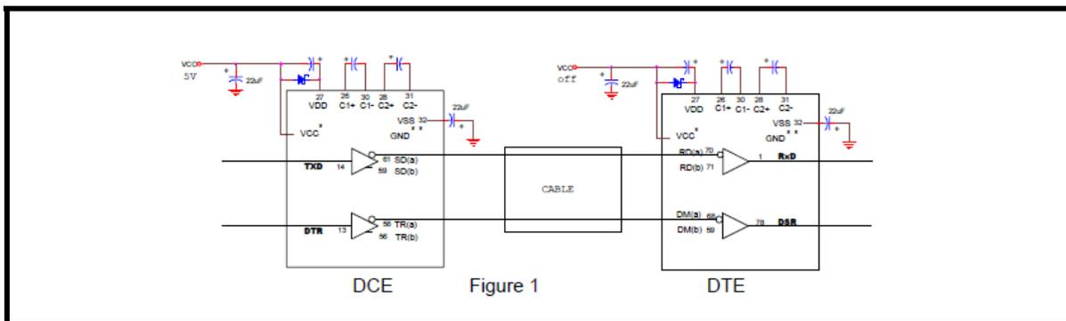
To create the latch condition the DTR line of the DCE SP507 Receiver input is a logic 1 which translates to the TR(a) output being -9V and the TxD line is a logic 0 with the SD(a) output at +9V. These voltages are then present on the un-powered DTE SP507 Receiver inputs DM(a) and RD(a) respectively.
