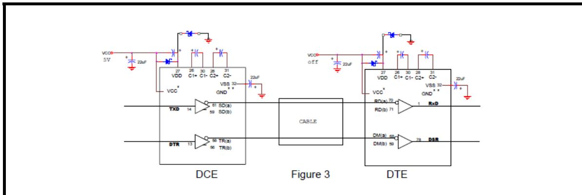
The anode of the Schottky is tied to ground and the cathode to Vdd
